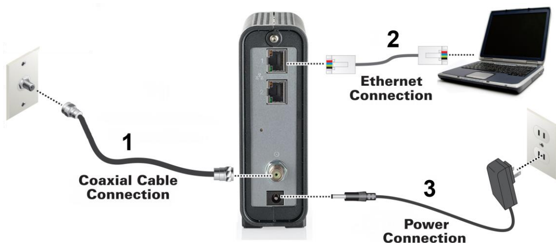
Figure 4: CM8200 Connection Diagram
